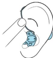
5. The wire is bendable closest to the top of the hearing aid and can be adjusted for comfort, retention and visibility.
