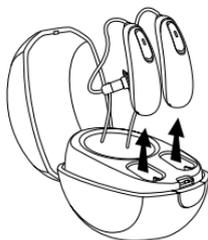
By default, the hearing aids are programmed so that they turn on automatically when they are removed from a charger that is connected to the power supply. Your hearing care professional can turn this setting off. In this case, you will need to switch the hearing aid on manually.
