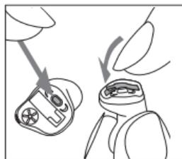
To enter flight mode press the push button for 7 seconds while closing the battery door. To exit flight mode, simply open and close the battery door again.
