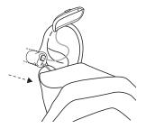
Using your thumb and index finger, gently pull the earmold (not the hearing aid or the wire) loose from your ear. If your earmold has a removal cord, pull it gently to assist. The removal cord is a separate line that is additionally attached to the earmold if requested. Remove the earmold completely by twisting it gently.
