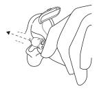
Hold the earmold between your thumb and index finger and position the sound outlet into your ear canal.
