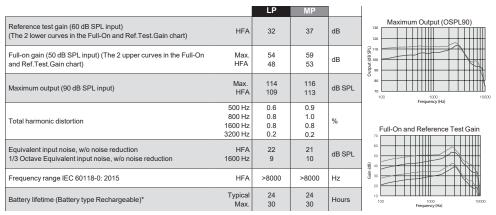
Measured according to ANSI S3.22-2014, IEC 60118-0:2015, JIS C 5512: 2015, 2cc coupler.
